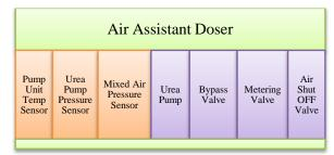
Fig. 3. Block diagram of Air Assistant Doser
